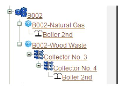
The Facility Tree should mimic the airflow as it is conveyed from the emission unit/process to the control device(s) (if any) and out the egress point(s).
